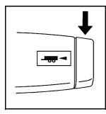
Pressing this button at the end of the shift lever turns on and off the tow/haul mode.
